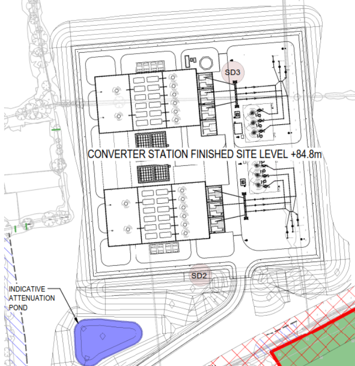
Plate 4 – Karst Features, Converter Station Layout Option B(ii) (Karst Features shown in pale red circles)
